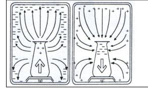
This charging frequently appears in heated rooms with dry air (less than around 40% relative humidity) and with weighing samples made of glass or plastic.
