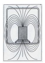
The magnetism of a weighing sample can lead to the weighing result being dependent on the position of the weighing sample on the weighing pan and to a result that is difficult to reproduce.
