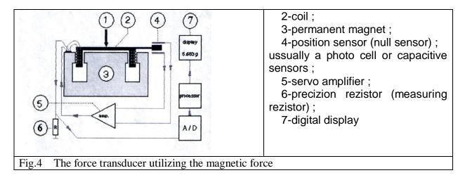
The force on the weighing pan is compensated by the permanent magnet and the magnetic field generated by the currentin the coil. This current is regulated by the sensitive position sensor and the servo amplifier, and mesured over the precision rezistor by the analog-digital converter. The balance measures the current needed to keep the pan in its position and the pan does not move. [2]
